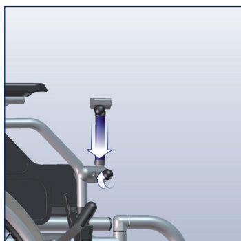
Attach the operating unit holder (5).
