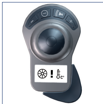
Warning notice Temperature Drive wheels
