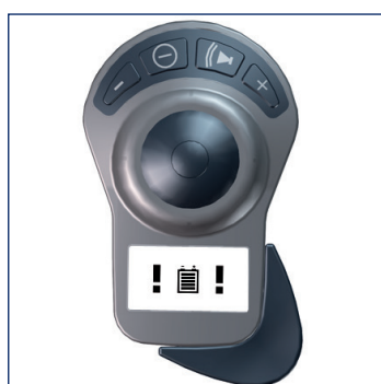
Warning notice Overvoltage Battery pack
