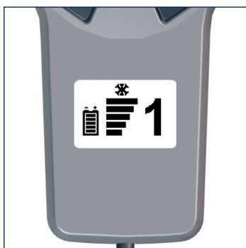
Standard display (when switched on with button 1) » Hill assist » Driving program 1 » Assistance level » Battery capacity
