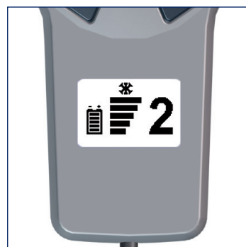
Standard display (when switched on with button 2) » Hill assist » Driving program 2 » Assistance level » Battery capacity
